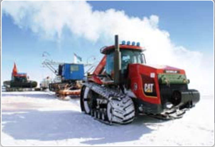
A Challenger MT800B Series tractor, owned by the U.S. government’s National Science Foundation, pulls a large bladder full of fuel as part of the South Pole traverse, a tractor-train hauling cargo from McMurdo Station to Amundsen-Scott South Pole Station.
